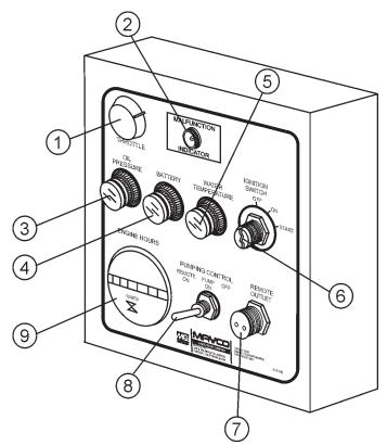
Figure 8. Pump Control Box Components
